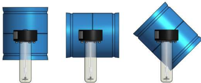
Fig. 3 Examples of installation
